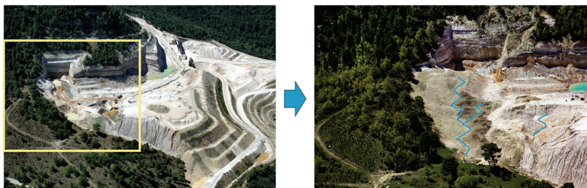
Figure 7. Left, oblique aerial view of the area of El Machorro mine where the GeoFluv reclamation is starting to be applied. This picture show the traditional terraced reclamation approach —with the experimental area in the lower right corner— and the beginning of the GeoFluv reclamation works. Right, image covering the area of the yellow rectangle of the left that shows an already reclaimed area (central zone, with brown-ocher colors and blue line of fluvial network), blended with the natural surroundings (to its left); the short blue line to the right shows the area where the reclamation is continuing, in this case excavating a valley in the pre-existing terraced spoil heap.
